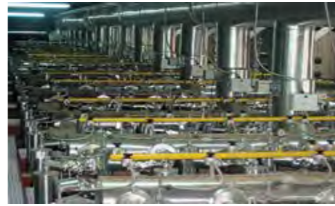
Tunnel kiln fired with preheated combustion air from cooling zone saving 50kJ/kg
